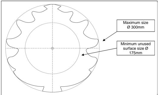
Please note that the same conditions apply for shaped picture discs as they do for standard ones (risk of moiré, warping on single sided picture discs, degraded acoustic quality).
